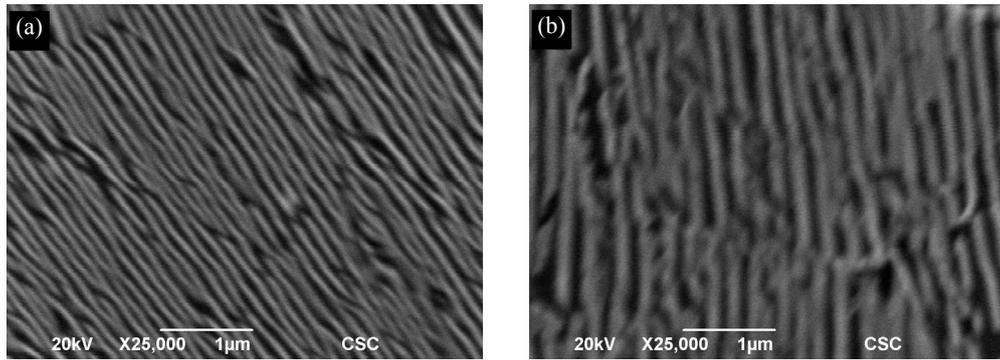
Fig.6. SWRH62A inter-lamellar spacing of SEM samples (a) standard cooling, 75nm (b) slower cooling, 105nm.
