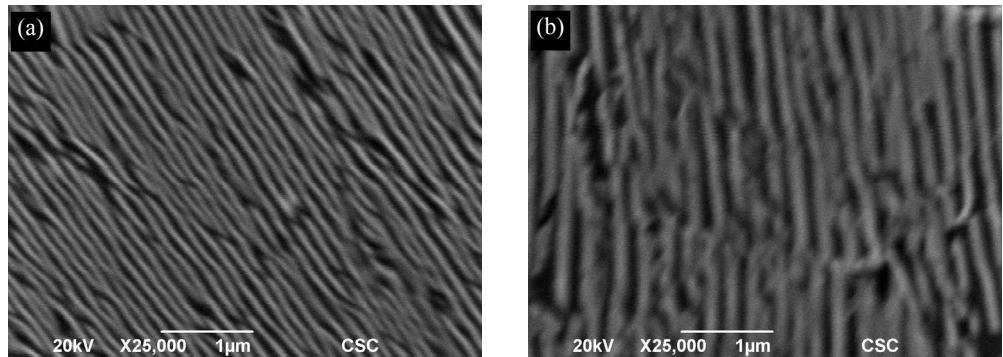
**Fig.6.** SWRH62A inter-lamellar spacing of SEM samples (a) standard cooling, 75nm (b) slower cooling, 105nm.
