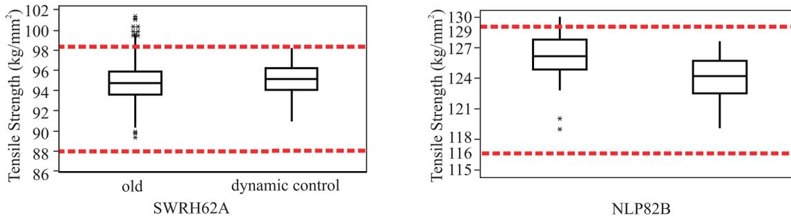
Fig.8. Box plot of TS after applying dynamic control technology.
