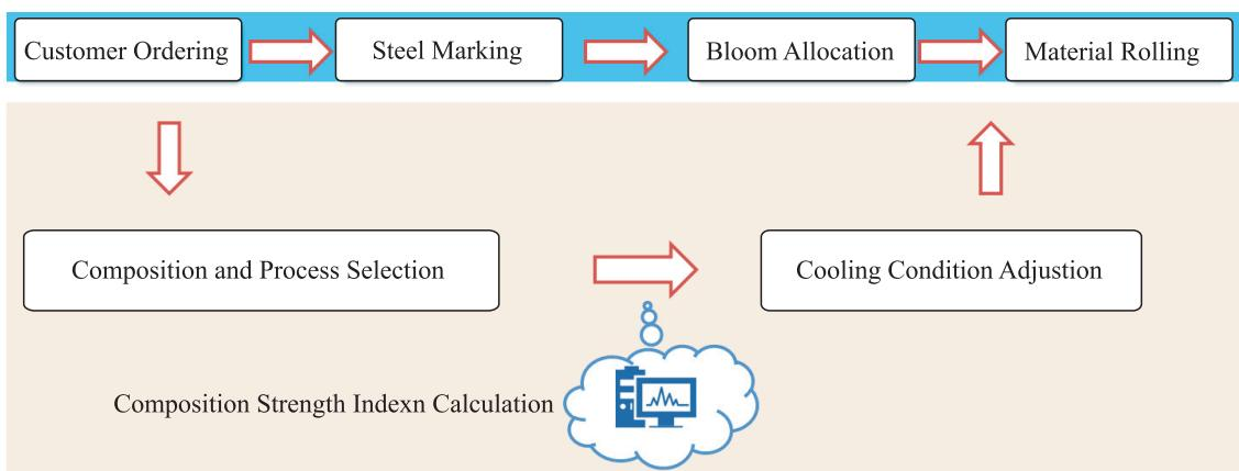
**Fig.7.** Schematic of wire rod production.
