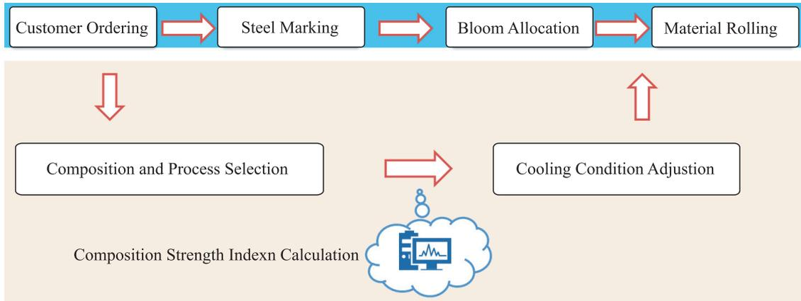
Fig.7. Schematic of wire rod production.
