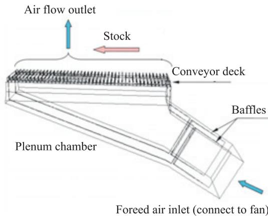
**Fig.2.** Assembly of a single plenum Stelmor air conveyor system.
