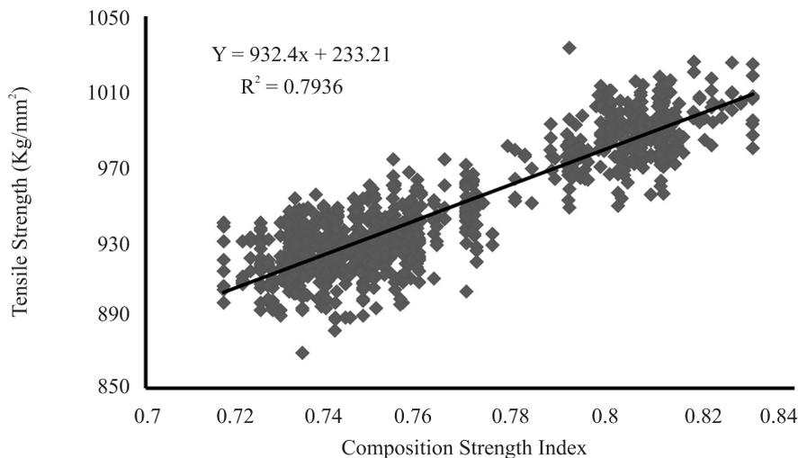
Fig.4. The correlation of SWRH62A between CSI and TS.
