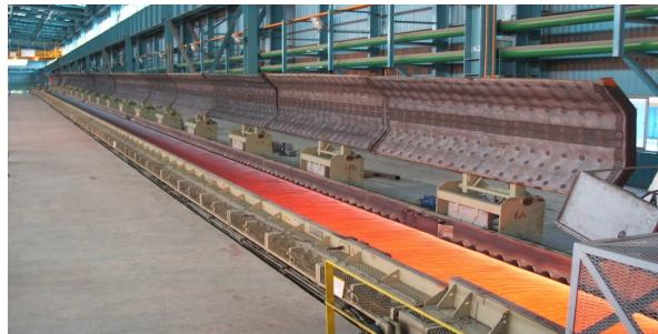
**Fig.1.** The Stelmor conveyor in the ROD2 Mill at CSC.
